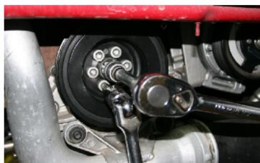
good quality 6mm hex key, one that has no wear on the points or you may round the bolt sockets. Take care when undoing these bolts, as they can be quite tight and can be easy to round. If the bolt shows signs of starting to round before you can loosen it, try a product that freezes the bolt to help loosen it.
