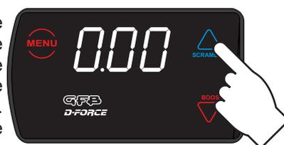
If you want to activate scramble using a remote-mounted button, switch, warning light, ECU output etc, you first need to connect the blue remote wire to the button/switch/ECU output you want to use (see page 4 for wiring diagram), then set the input to “SCr” (see page 15, “Auxiliary Input Setup”). Once you have done this, the remote input will replicate the function of the up/scramble button, and the up/scramble button will also change colour in the same way to indicate when scramble is active.
