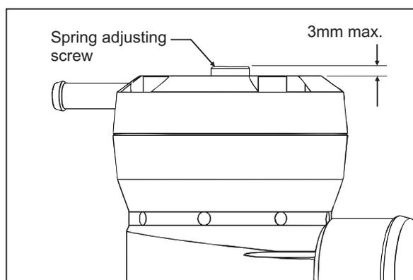
It is possible to use the Mach 2 straight out of the box without any spring pre-load adjustments, however you can use the adjustment to fine-tune throttle response. Generally speaking, the hardest spring pre-load you can run without causing compressor surge (fluttering sound when lifting off the throttle) is ideal.
