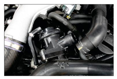
3) Fit the GFB Mach 2 value to the mounting flange, making sure the supplied red o-ring is fully inserted into the groove in the underside of the GFB value as shown below. Replace the two bolts, vacuum and recirc hoses and clamps.
