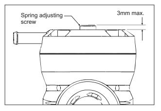
The recirc versions of the Mach 2 are supplied with GFB's softer spring (part # 6116), which cannot be used for atmosphere venting because the piston will usually hover slightly open at idle (similar to the factory valve).
