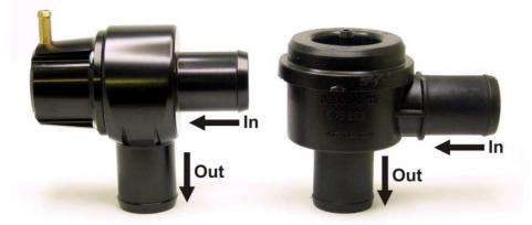
You can easily check for the correct orientation by tracing the 2 large diverter valve hoses – the bottom inlet of the dv+ connects to the intercooler piping, and the side outlet connects to the turbo intake.
