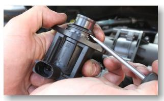
3. Remove the second yellow o-ring and keep it handy, as these will be used in the DV+ assembly.
