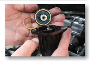
4. Assemble the GFB parts onto the factory solenoid body as shown in the exploded view below, making sure to use the GFB-supplied plunger spring, and the two yellow factory o-rings.
