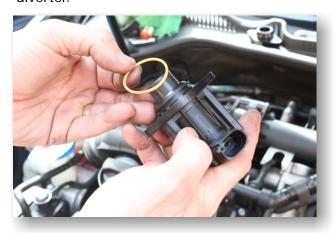
2. Using a flat screwdriver in the o-ring groove, carefully pry the piston surround from the solenoid body.
