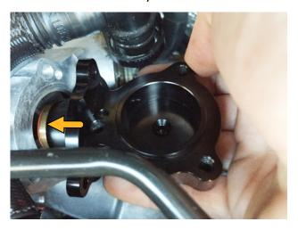
Insert the GFB plunger spring into the diverter solenoid, followed by the plunger. Put the yellow factory o-ring on top of the DV+ body. Hold the plunger with your finger and fit the solenoid assembly onto the DV+ body.
