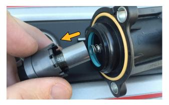
Remove the plastic piston shroud from the solenoid. This should be able to be removed by hand, but if it does need to be levered out take care not to damage any of the plastic pieces. Store the piston, shroud and spring safely as these are not used, and keep the yellow o-ring and bolts for the DV+ installation.
