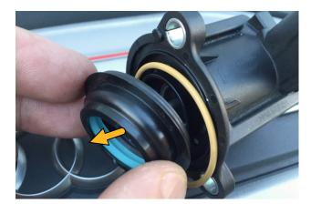
Check the fit of the piston in the DV+ body. It is a very tight tolerance and can sometimes be tricky to get started into the bore. Once inserted, it should slide freely without sticking.
