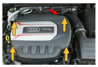
Unclip the breather pipe (red arrow) and diverter valve electrical connector (yellow arrow), then loosen the hose clamp and remove the intake pipe (white arrow).
