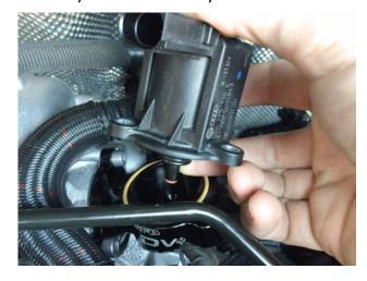
Fasten the solenoid using 3 screws (GFB or factory screws, they are the same). Re-install the turbo intake elbow, intake pipe, breather hose, and electrical connector in the reverse order of disassembly.
