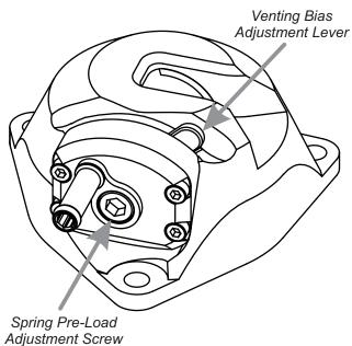
hard rev - stab the throttle hard and release quickly. The piston should lift quickly and vent, then close slowly and smoothly. The harder you stab the throttle, the further the piston will open.
